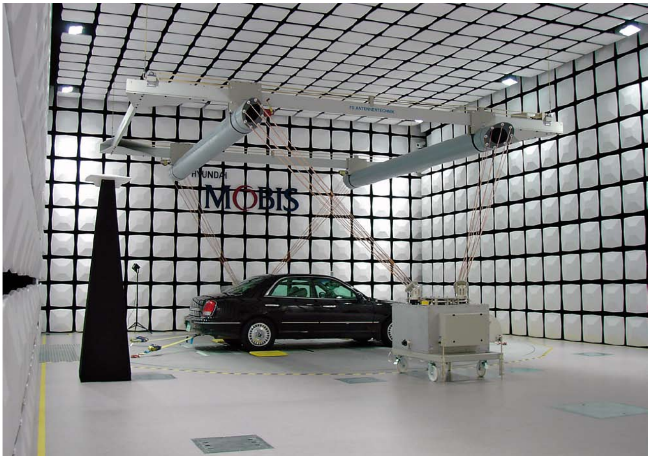
FIG 1 Modern anechoic chamber with E/H field generators above vehicle. Rohde & Schwarz supplied the complete EMC measurement equipment for this chamber.
