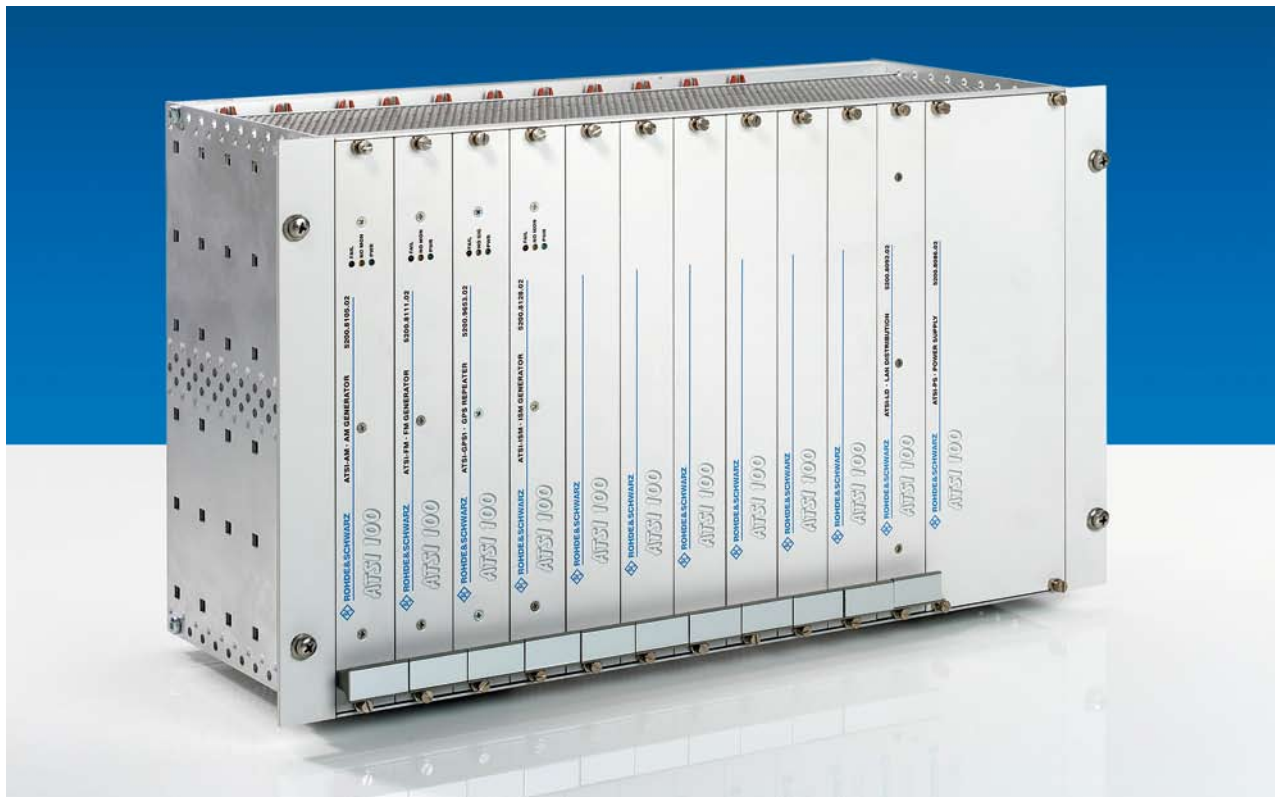
FIG 2 Function modules of the R&S®ATSI infotainment test system in the rack.
